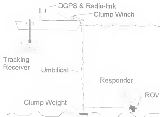
FIG. 2. Schematic diagram showing the method of anchoring a 20 m vessel over the study sites and deployment of the ROV on nylon rope.
